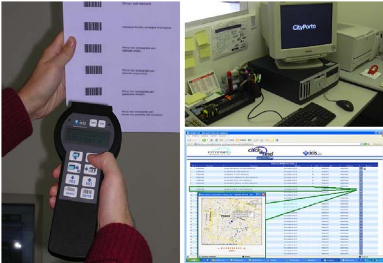
The main components of Cityporto's tracking system.
