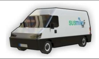
Capacity: maximum between 1200 kg and 1500 kg Power options: Fossil fuels / alternative fuels (gas, electric)
